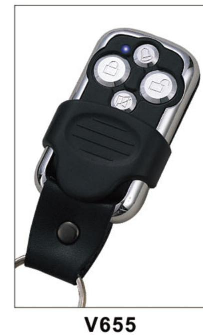
Product name: Duplicable Remote Control model No.: V655 **Brand Name: VICTOR** Packing:25PCS/BOX Configuration Files: Adjustable Frequency Technical Parameter: ASK Packaging Parameter: 500PCS/CTN Frequency:(301MHZ-503MHZ)
