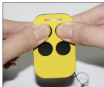
2. To remove the existing code: Press 1st button and 2nd button until the LED flashes (approximately 10 seconds), release both buttons and all codes will be eliminated.
