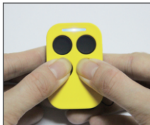
4. Code retrieval : If the code is inadvertently removed The previous code can be retrieved by 3rd button and 4th button until the LED flashes (approximately 5 seconds)
