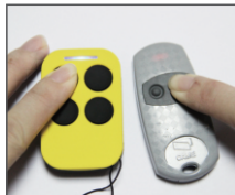
3. To duplicate code: Hold the original duplicator as close as possible to each other. Press 1st button on both duplicator and original transmitter at the same time, after 3 seconds, the LED will flash steadily, release both buttons and the code will have been accepted. Repeat the above operation to duplicate the code of the other buttons.
