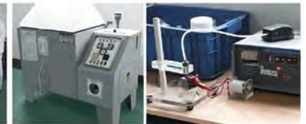
Salt spray test machine
