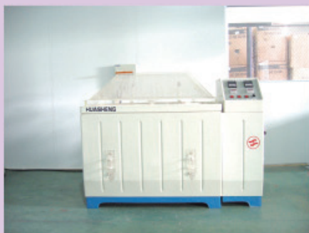
盐雾腐蚀试验箱 Corrosive salt spray chamber
