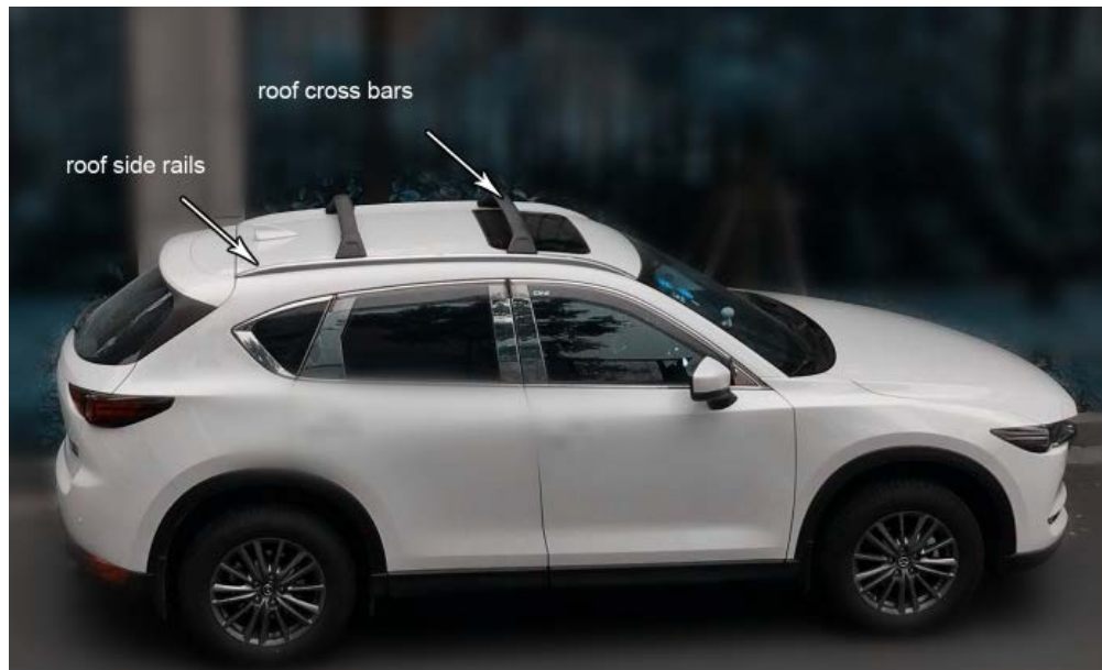
Item: 8153Y18-1 roof side rails aluminum base + aluminum bars silver color
