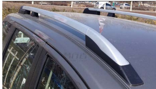
Aluminum and ABS car roof side rails
