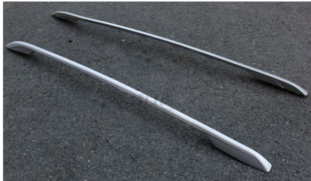
Roof side rails
