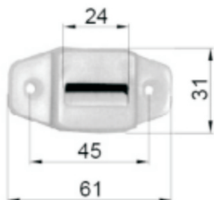
Guidacinghia Transversale per cinghino 23mm Waagerechte Leitrolle,FÜR gurt 23mm Strap Guide,horizontal,for strap 23mm 织带导轮, 23mm 宽织带用
