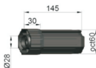
Calotta oct40 per cuscinetto Od28 Kapsel oct40 für Kugellager Od28 Plastic cap oct40 with bearing housing dia.28mm 塑料尾插, oct40,配OD28轴承
