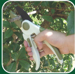
Anvil pruners: for cutting old and tough wood
