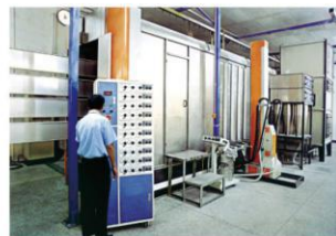
瑞士金马全自动喷涂生产线控制台 Switzerland Gema automatic painting production line control
