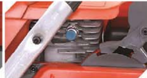
Decompression valve for easy start
