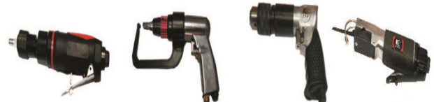
气动螺丝批 Grinding machine 定位点焊钻 Spot welding drill 气动钻 Pneumatic drill 气动锯 Pneumatic saw
