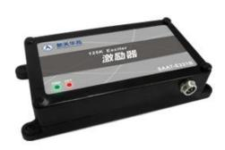
SAAT- E221B low frequency activator is an important component in active RFID system. SAAT-E221B sends LF signal to the standby status wake-up RFID tag and activates it. SAAT-E221B can activate the tags around it like a round area. With the help of Active RFID reader, LF Activator and LF& Active Wake-up RFID tag, this combination can realize the regional location and detect direction of movement. At the same time, the wake-up tag has longer battery life.
