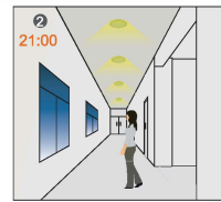
When motion detected, insufficient daylight, light ON.
