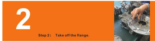
Step 2: Using Allen key(8mm) disassemble front cover, take down the Sealing paper pad.
