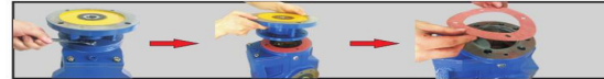
Step1: Using spanner(size:16) disassemble input flange, take down the Sealing paper pad.
