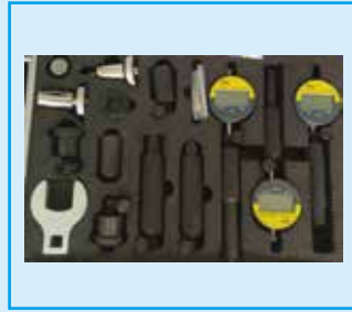
No,029(2) Common Rail Injector Valve Measuring Tool
