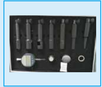
No,30(2) Common Rail Injector Valve Measuring Tool
