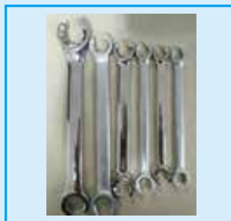
No,968 Disassembly Tools for Oil Pipe ( \phi 8 , \phi 9 , \phi 10 , \phi 11 , \phi 12 , \phi 13 , \phi 14 , \phi 17 , \phi 19 , \phi 21 )
