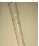
淋水管 Spray Pipe
