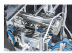
Three sides pre-heating system
