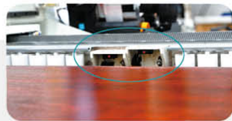
Two sensors: Double assurance to raise to the correct height
