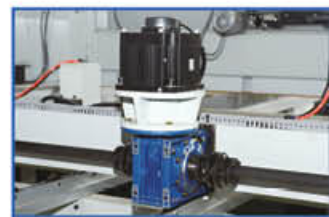
Italy Rack and Pinion Japan Mitsubishi Servo motor
