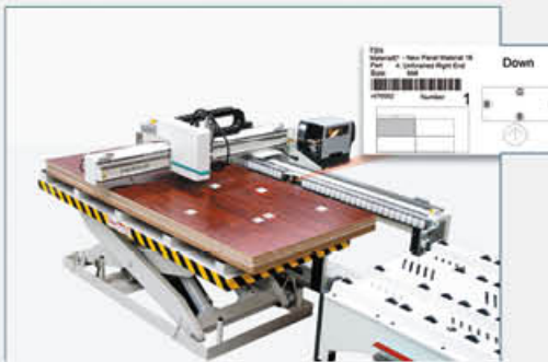
Pre-label device: Automatic and independent working
