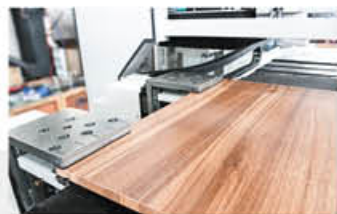
Grippers are automatically positioned to accommodate to different sized workpiece
