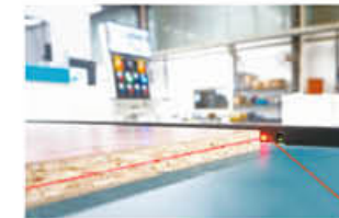
Sensor at the end of the unloading table avoids the workpiece running beyond the table
