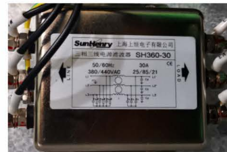
Three-phase three-wire power filter
